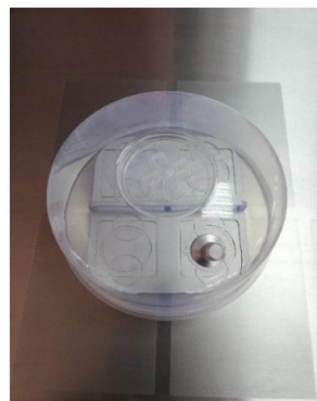
Figure 11.8 Gas hood placed over the gas nozzle
